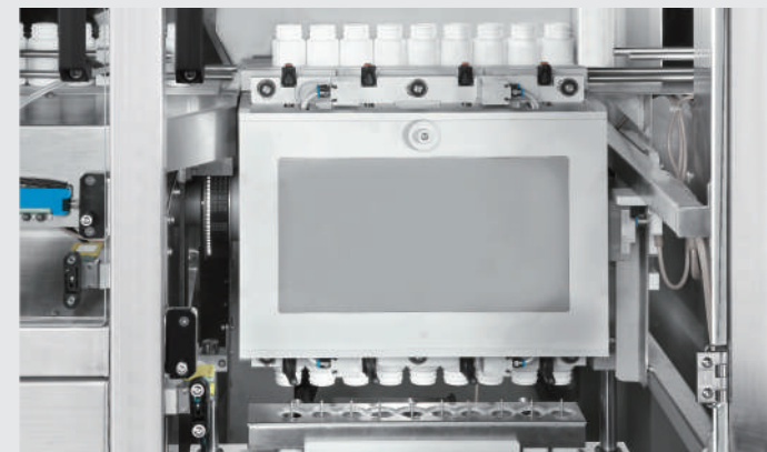
• Air Rinse Station
