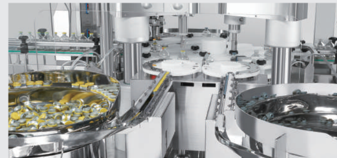
• Automatic unscrambling vibrators for rubber stoppers, plugs and caps.
