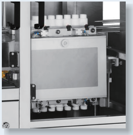
AIR RINSE STATION
